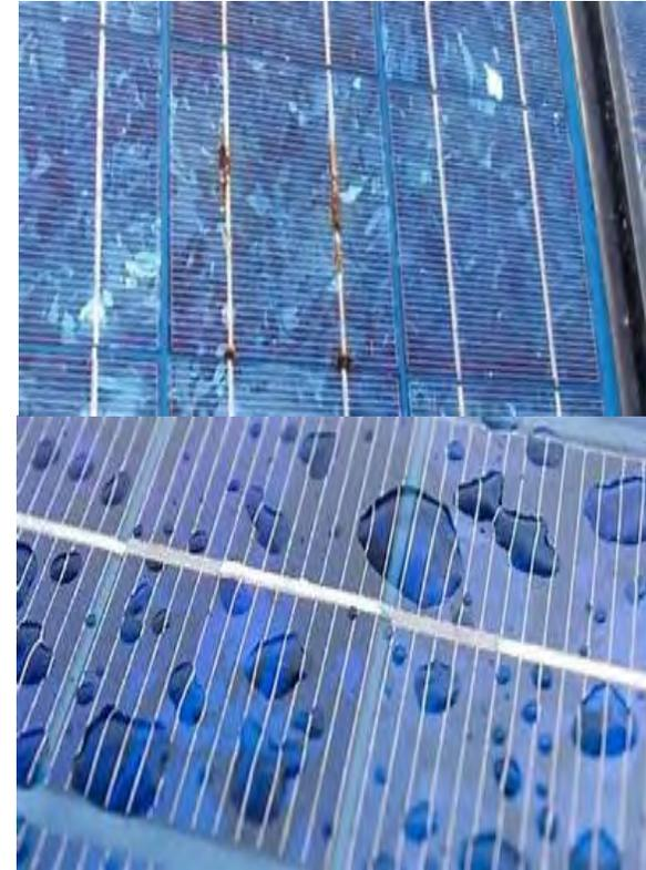
Fig 1: Moisture accumulation in SPV
